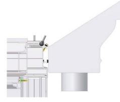
Place the guttering into position so that is sits tightly against the pivot channel of the Eaves Beam. Check the gutter for being level and square to the Eaves Beam.
