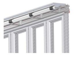
Clip the Eaves Beam packers (C9118) into position in the Eaves Beam Cover Adaptor (A5148) at approx 600mm centres.
