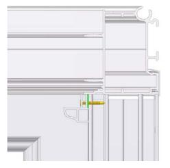
Fit the "Capella" soffit trims around the internal perimeter of the orangery (ensuring that the mitres are tightly together in the corners).
