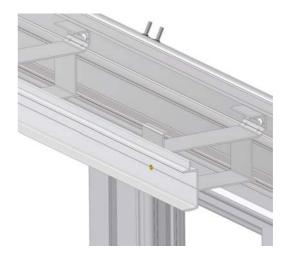
Continue to fix the adaptors around the internal perimeter, ensuring that the mitres are tightly together in the corners.
