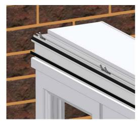
Ensure that the tape is firmly pressed into position prior to removing the protective film.
