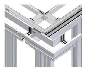
Place the Gutter Corner (with jointer) into position and is firmly bedded onto the silicone/Butyl tape joint. Clamp and compress the joint together prior to drilling and fixing.
