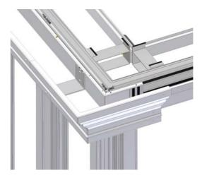
Working around the orangery, fix each joint using the same method. Clean off any excess silicone once permanently fixed together.
