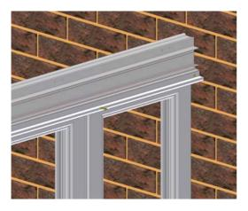
If not already fitted, fix the "Capella" soffit bracket (C9463) to the pre-drilled holes in the upper face of the Eaves Beam using the pop rivets supplied (C9480).
