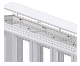
Position the back edge of the (175mm wide) upper Soffit Board (C9486) using the upstand on the top of the Eaves Beam.
