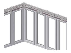
Once the soffit brackets installed, If not already fitted, fix the Eaves Beam Cover Adaptor (A5148). The adaptor should be centrally located into the recess on each bracket prior to fastening permanently using either pop rivets (C9480) or screws(C9489).
