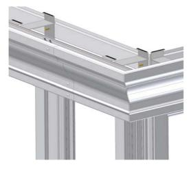
Fix the Gutter Corner to the Eaves Beam using the Gutter Fixing Screws (C9479) approximately 25mm from each end and in from the corner. Fix the "Capella" soffit trim (P6095) tight to the underside of the eaves beam and screw fix (C9489) to the inside face of the window (50mm from the ends and at approximately 450mm centres), ensuring that 1mm packers are placed between the trim and windows. It is recommended that the soffit trim should be pre-drilled with a clearance hole prior to installation.
