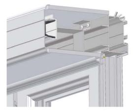
When fitting the Eaves Beam Cover (P6042) ensure that a gap is present in the corners to allow fitting of the Internal Eaves Cover Joint Trim (C9108). Push fit the joint trims into place.
