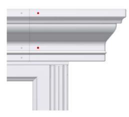
Mark the drilling positions. It is important that the drilled holes pass through the silicone filled channel between the Butyl Tapes and the jointer.
