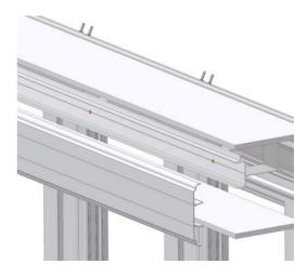
Check along the length of the Internal Eaves Beam Cover (P6042) to ensure that it has correctly located into the adaptor (A5148), if any adjustments are required, gently squeeze the top and bottom of the Eaves Beam Cover (P6042) and place in position before releasing.
