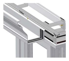
Once the tapes are pressed firmly into position, apply a liberal amount of silicone between the Butyl Tapes so it sits proud (no excess silicone is to be removed at this point).
