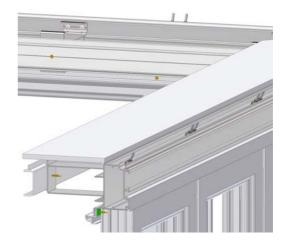
Fit the upper soffit claddings around the internal perimeter of the orangery, ensuring that the mitres are tightly together in the corners.
