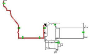
When riveting the back face of the gutter, ensure that it is riveted from inside.
